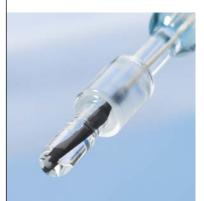
SevenExcellence offers the possibility to check the performance of a pH sensor. The special method type sensor test guides the user through the individual steps, checking various measurement characteristics of a sensor, such as drift and repeatability.
